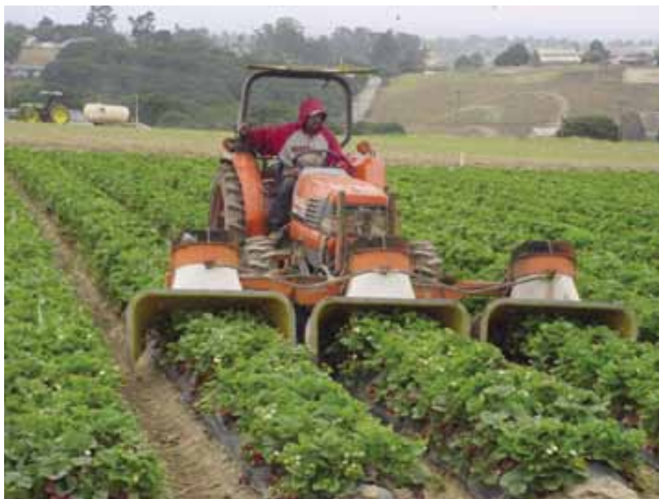
A Bug-Vac moves through a strawberry field. Aphids and other small, winged insects can move into organic fields and quickly reach damaging levels. Machines have been developed that use suction to capture and remove these insects.
