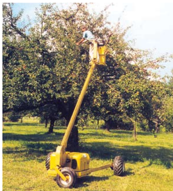
Safer and more practical than traditional ladders, hydraulic ladders are economically viable for maintenance and harvesting in large orchards.
